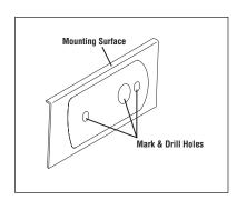
Remove the foam adhesive backer and drill two 3/8" and one 5/8" mounting holes in the marked positions.
